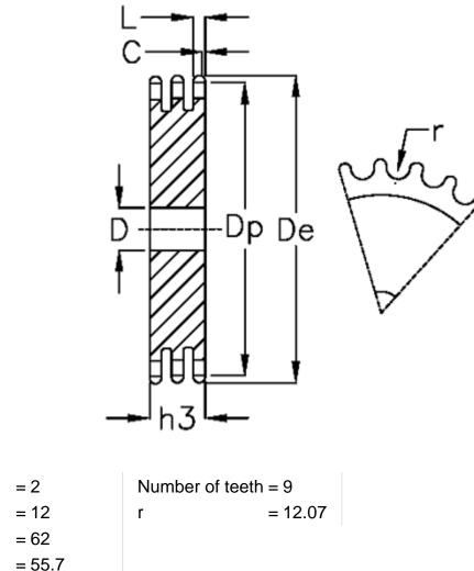
C = 2 D = 12 De = 62 Dp = 55.7 For chain size =  $3/4 \times 7/16$ For chain type = 12 B-3 h3 = 49.8 L = 10.8
